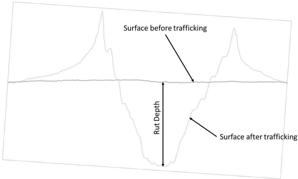
**Figure 8. Cross-section of rut showing rut depth definition.**
