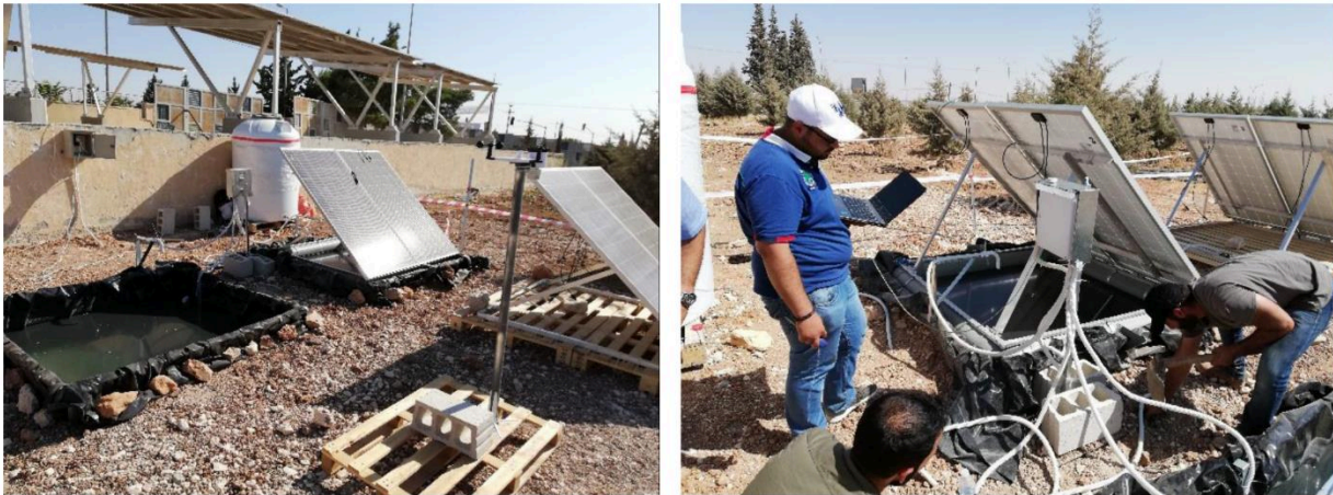
Figure 4. The pilot setup for evaporation reduction by floating solar panels study (Left), and the measurement system (data logger, ultrasonic, and temperature sensors) (right)
