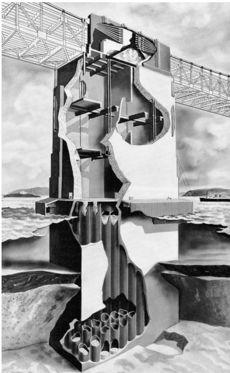
Figure 4-24. Middle anchorage W4 of San Francisco-Oakland Bay Bridge. Source: U.S. Steel (1936), with permission of American Bridge Co.
