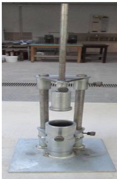
FIG. 2. Modified Harvard compaction equipment.
