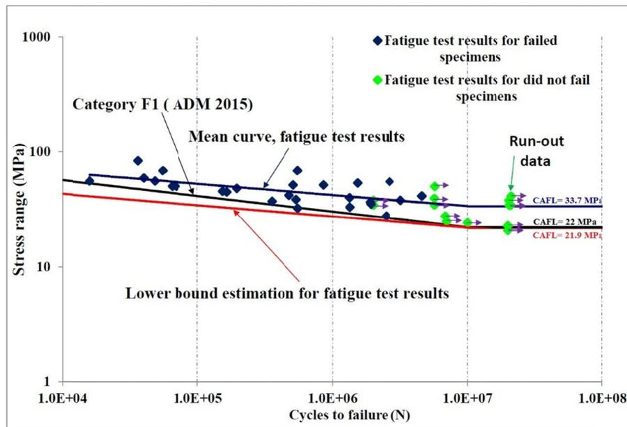
Fig. 8. Fatigue test results shoe base.
