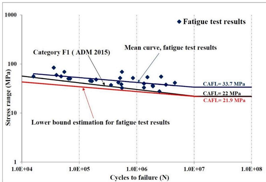
**Fig. 7.** Combination of best fit, lower bound estimation, and category F1 S-N curve.
