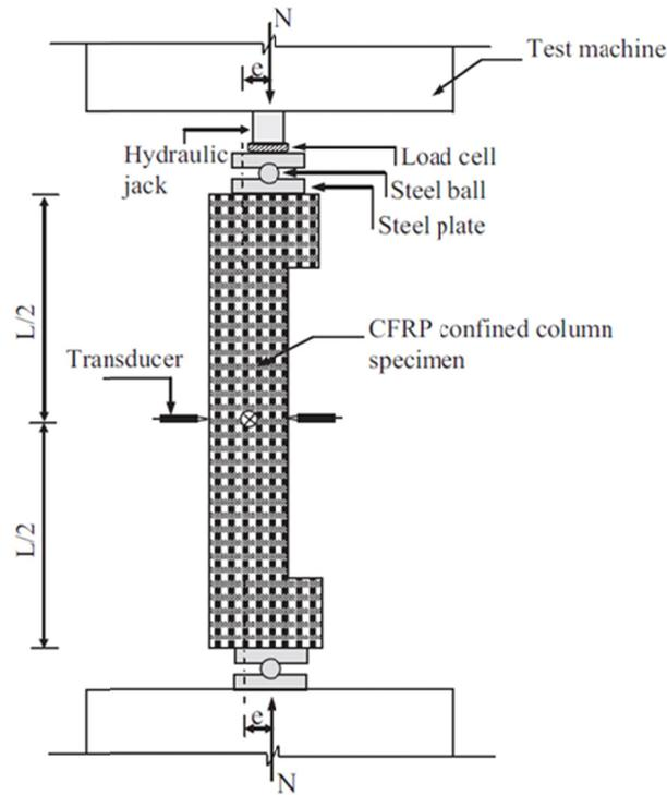
Figure (5): Experiment setup, Figure from (Dundar et al., 2015).
