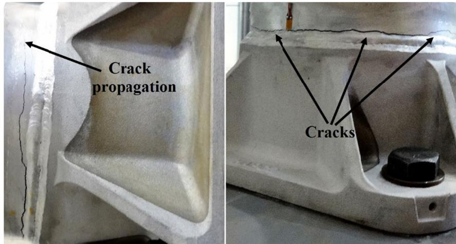
**Fig. 5.** Crack propagation in the specimens. (Photograph courtesy of testing engines and structures center, The University of Akron, Akron, OH)
