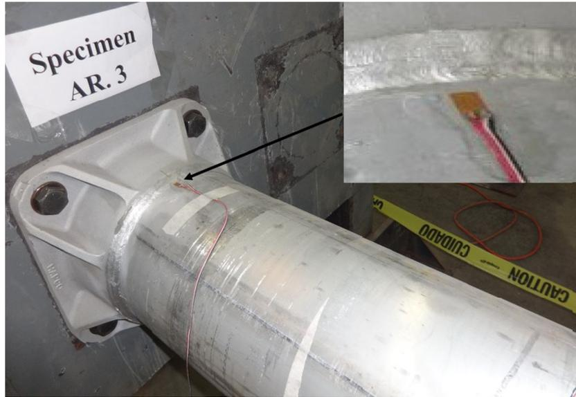
**Fig. 4.** Position for strain gages. (Photograph courtesy of testing engines and structures center, The University of Akron, Akron, OH)
