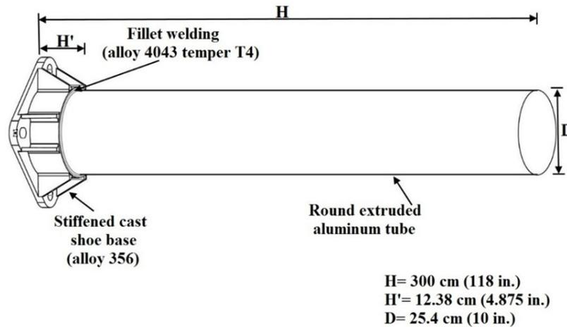
**Fig. 2.** Shoe base light pole dimensions for fatigue design.
