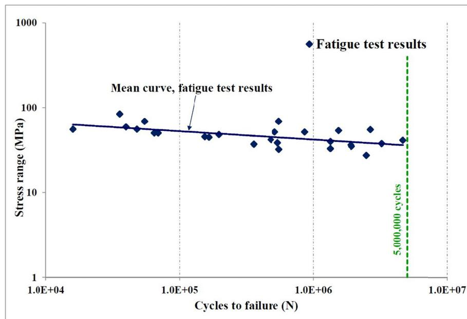
**Fig. 6.** Failure data for shoe base light poles.
