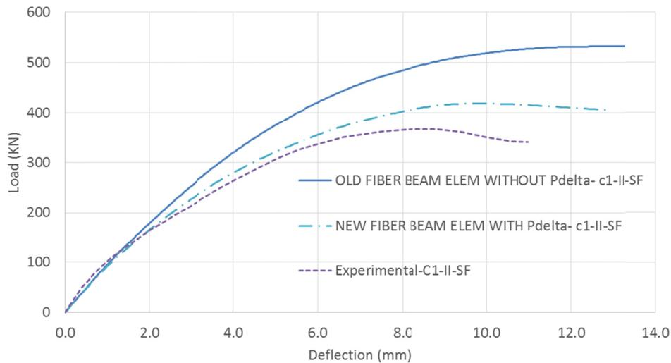
Figure (6): Load-deflection curve for column C1-II-SF tested by (Dundar et al., 2015) and compared with the new and old fiber beam elements.
