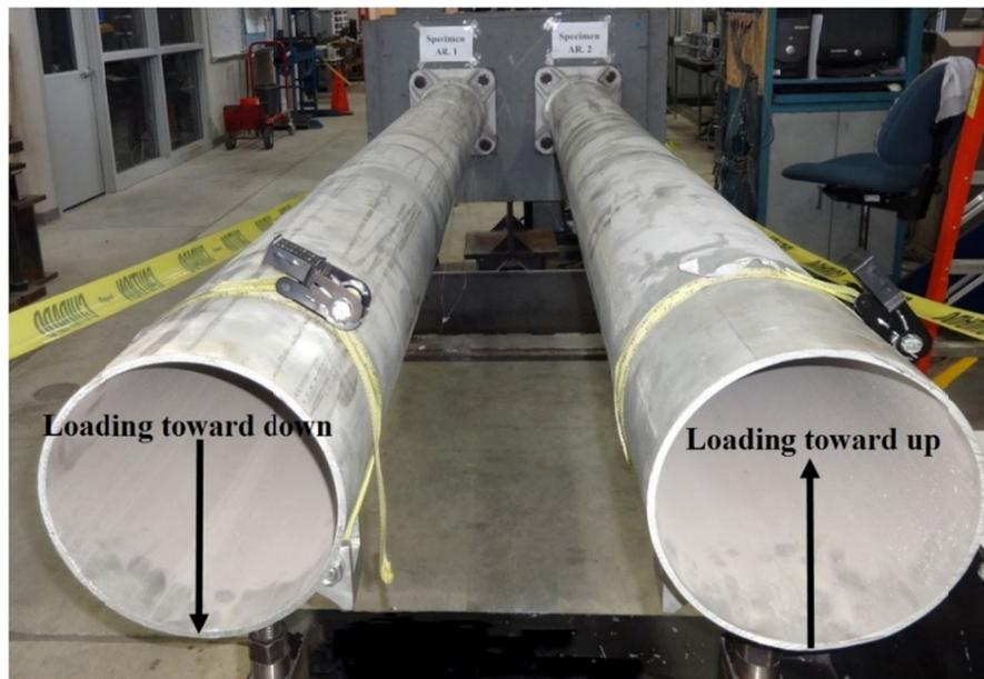
**Fig. 3.** Fatigue testing device for two specimens together. (Photograph courtesy of testing engines and structures center, The University of Akron, Akron, OH)
