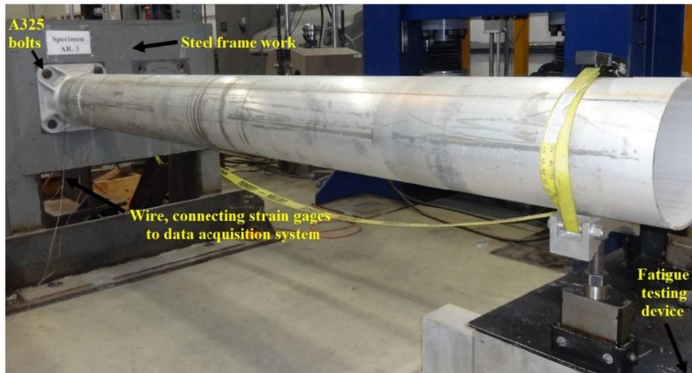
**Fig. 1.** Shoe base aluminum light pole. (Photograph courtesy of testing engines and structures center, The University of Akron, Akron, OH)
