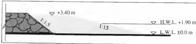
Fig. 3. Typical design cross section of the beach
