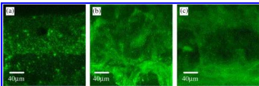
**Figure 16.20** CLSM images of biofilms formed on the hollow fiber: (a) aerobic MBR at 2 kPa, (b) aerobic MBR at 30 kPa, (c) anoxic MBR at 30 kPa (adapted from Yun et al., 2006).
