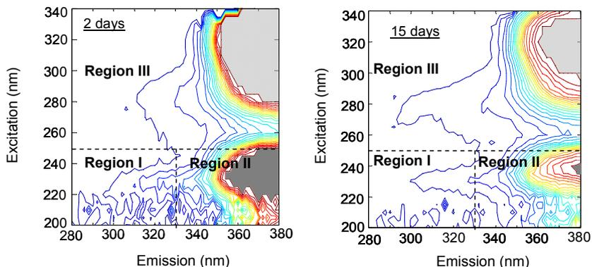
**Figure 16.19** EEM fluorescence spectra of membrane foulants collected on 2 days and 15 days of operation (adapted from Aryal et al., 2009).
