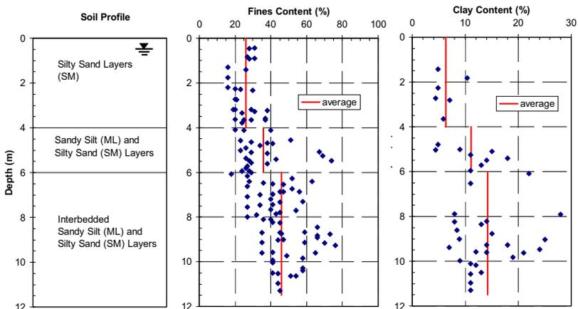
FIG. 1. Idealized soil profile along with fines content and clay content profiles.
