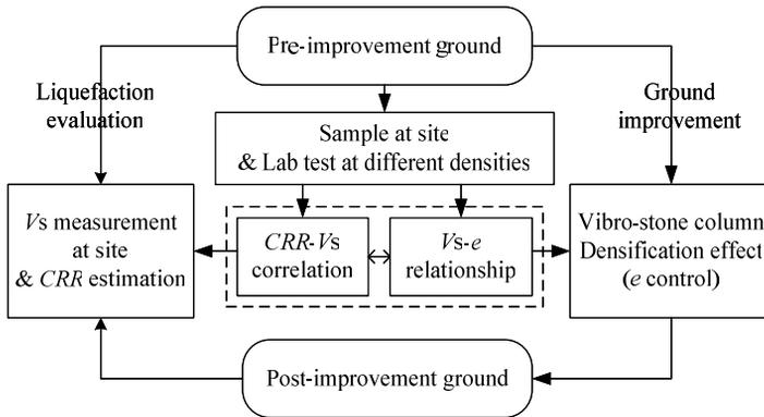
FIG. 3. Flowchart for evaluation of ground improvement by shear wave velocity.
