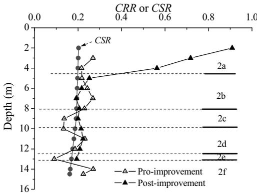
**FIG. 6. CRR estimation based on shear wave velocities.**
