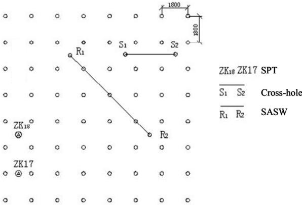
FIG. 4. Layout of seismic wave and SPT tests.
