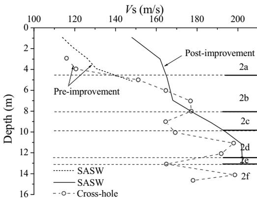
FIG. 5. SASW tests before and after ground improvement.
