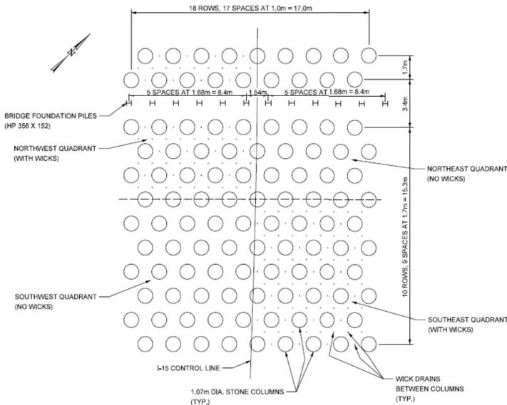
**FIG 3. Layout of stone columns and wick drains.**
