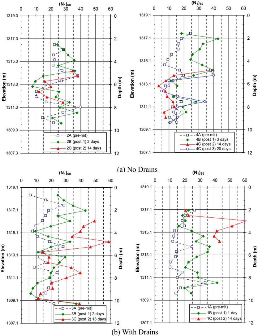
**FIG. 2. Results from SPT testing in (a) two test areas without wick drains and (b) two test areas with wick drains during stone column treatment.**
