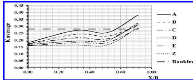
FIG. 12. Values of  $K_{av}$  vs. X/B for different soil stiffness and  $t/H = 0.1$
