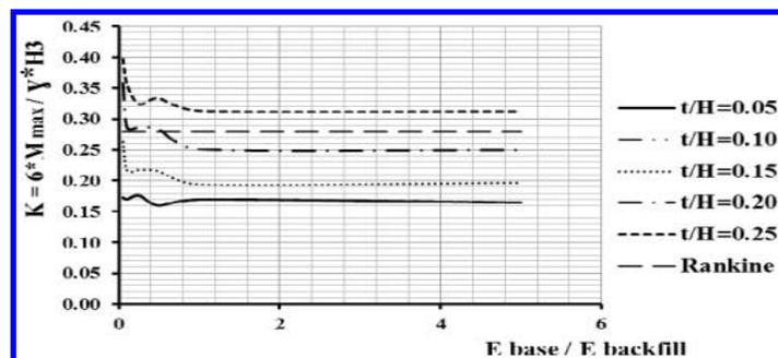
FIG. 13. The values of K vs. soil stiffness ratio for different t/H and X/B = 0.71
