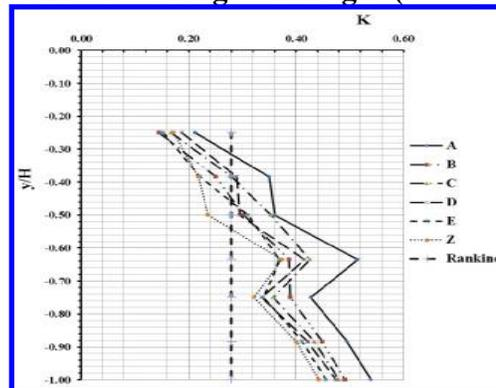
FIG. 8. Dist. of EP coefficient (K) along wall height ( $t = 0.40$  m and  $X/B = 0.71$ )
