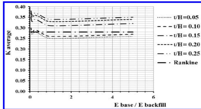
FIG. 9. Values of  $K_{av}$  vs. soil stiffness ratio for different  $t/H$  and  $X/B = 0.71$
