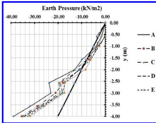
FIG. 7. Lateral EP dist. along wall height ( $t = 0.40$  m and  $X/B = 0.71$ )
