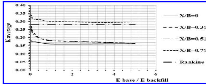
FIG. 11. Values of  $K_{av}$  vs. soil stiffness ratio for different X/B and  $t/H = 0.1$
