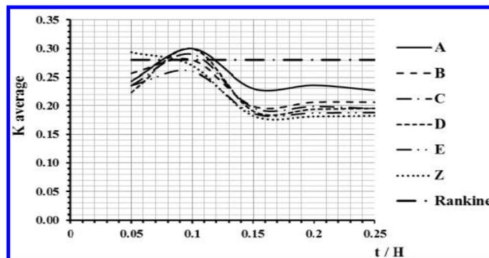
FIG. 10. Values of  $K_{av}$  vs. ratio ( $t/H$ ) for different soil stiffness and  $X/B = 0.71$
