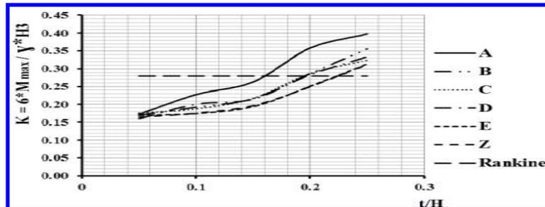
FIG. 14. The values of  $K$  vs. thickness ratio for different soil stiffness,  $X/B = 0.71$
