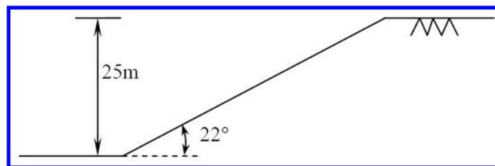
**FIG. 1 Cross Section of a homogenous  $c-\phi$  slope**
