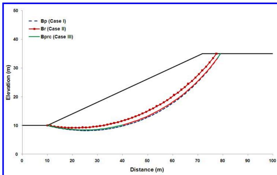
FIG. 2. Deterministic critical slip surfaces for Case I, Case II and Case III
