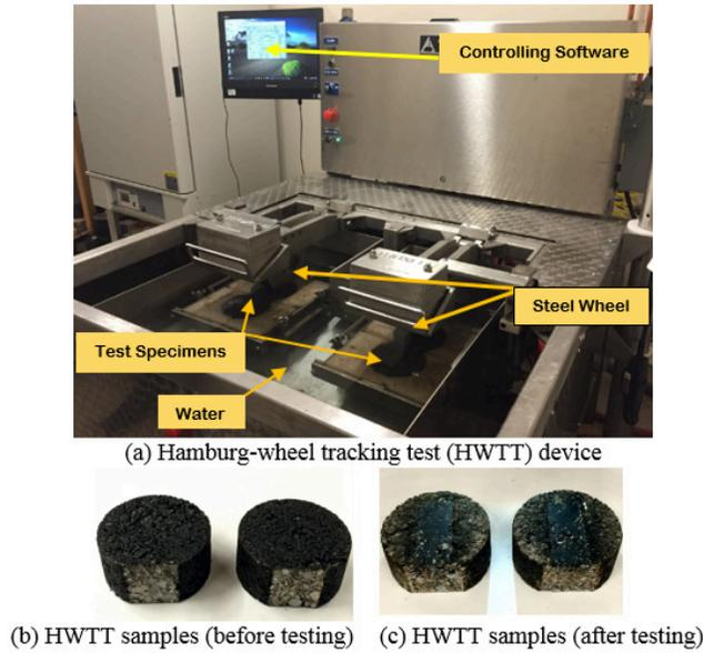
**Figure 2: Hamburg-wheel tracking test device and samples.**
