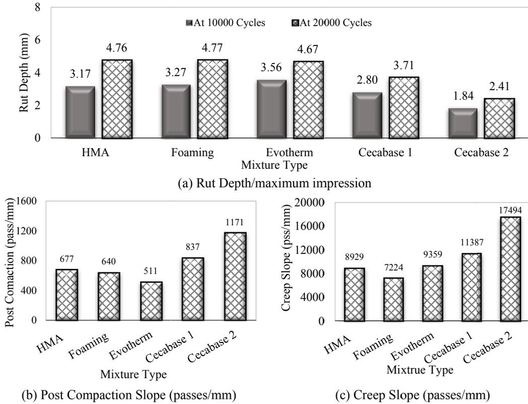
**Figure 6. Plot of rut depth, post compaction slope, and creep slope analysis.**
