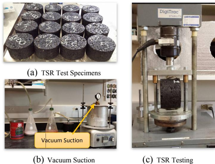
**Figure 4. Tensile strength ratio (TSR) test.**
