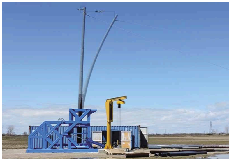
Figure 5-2. Vertical full-scale test fixture based on ASTM D1036-98 principles. Source: Courtesy of RS Technologies Inc.
