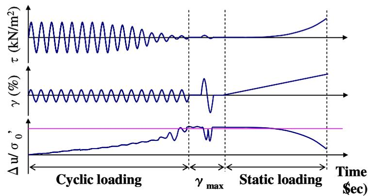
FIG. 2. Pattern diagrams of loading process
