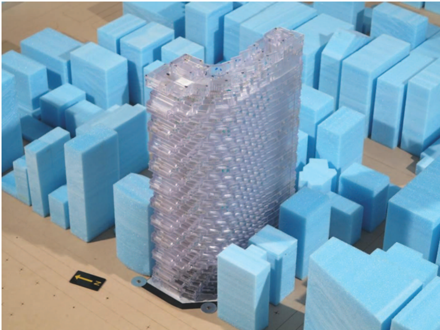
Figure 6-2. High-frequency pressure integration model: Torre Shyris 18, Quito, Ecuador.
