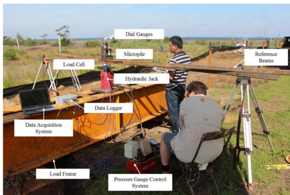
Figure 2. Set-up for pullout testing
