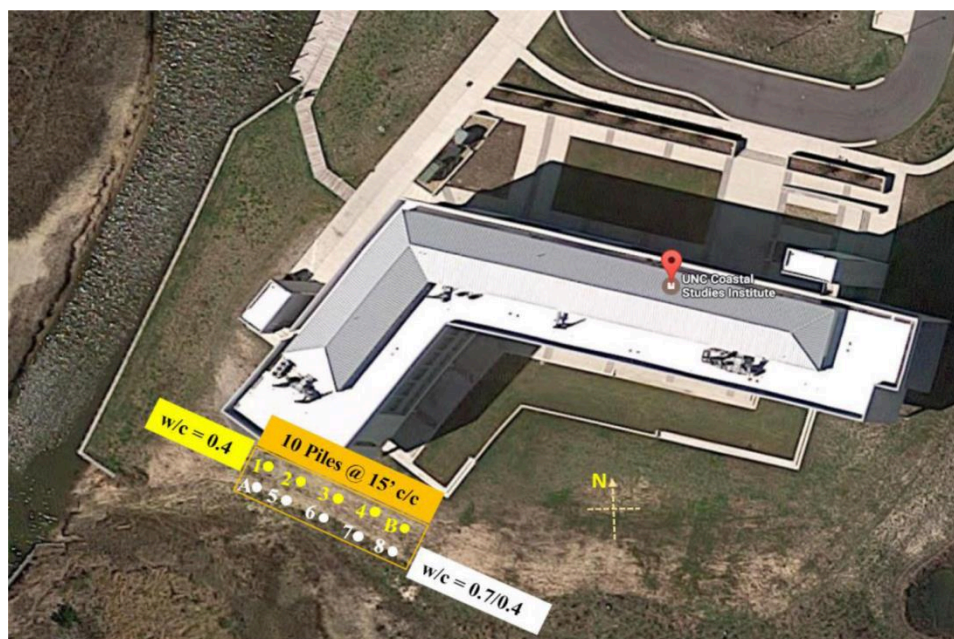
Figure 1. Field deployment of ten micropiles
