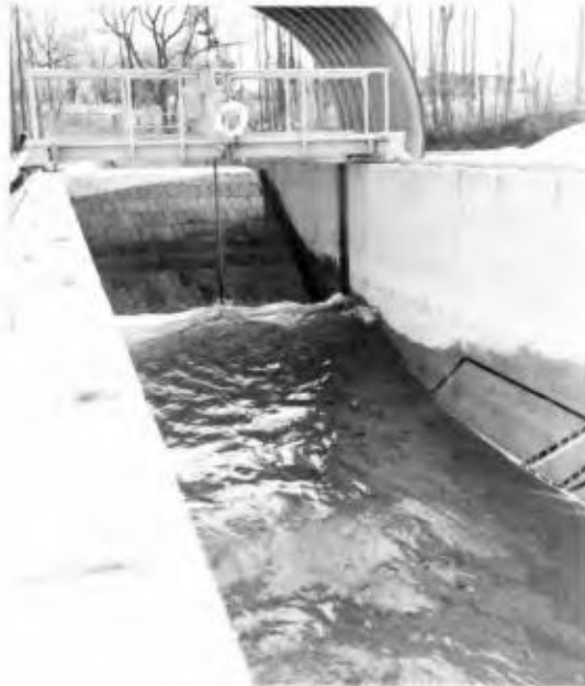
Fig. 7. Concrete block revetment in large wave tank.
