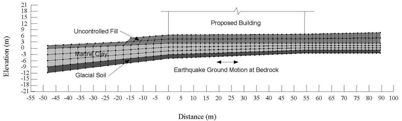
**Figure 4. Finite element model of east-west section**
