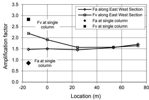
Figure 13. Site coefficients  $F_a$  and  $F_v$  from modified Northridge 1994
