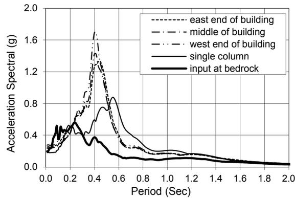
**Figure 6. Response spectral acceleration from modified El Centro 1940**
