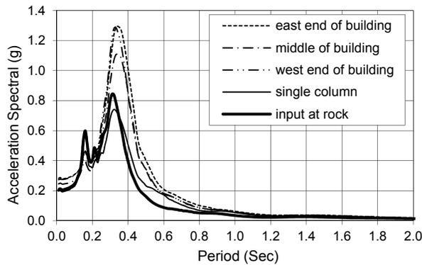
Figure 10. Response acceleration spectral from modified NH Franklin Falls Dam 1982
