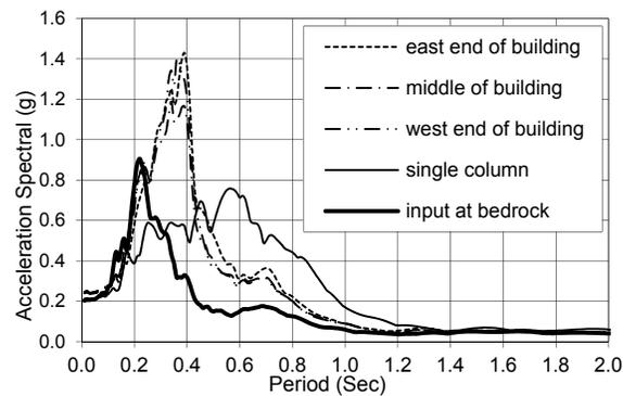
**Figure 8. Response spectral acceleration from modified Northridge 1994**
