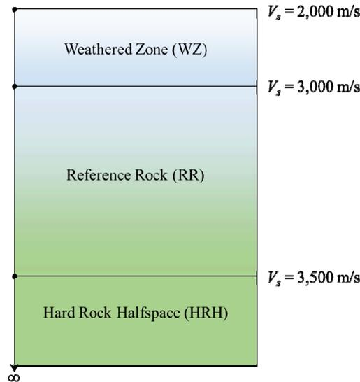
**Figure 1. Schematic of reference rock and weathered zone velocity model (not to scale).**
