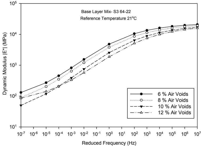
Figure 1 Master Curves for Base Layer Mixes (S3 64-22)
