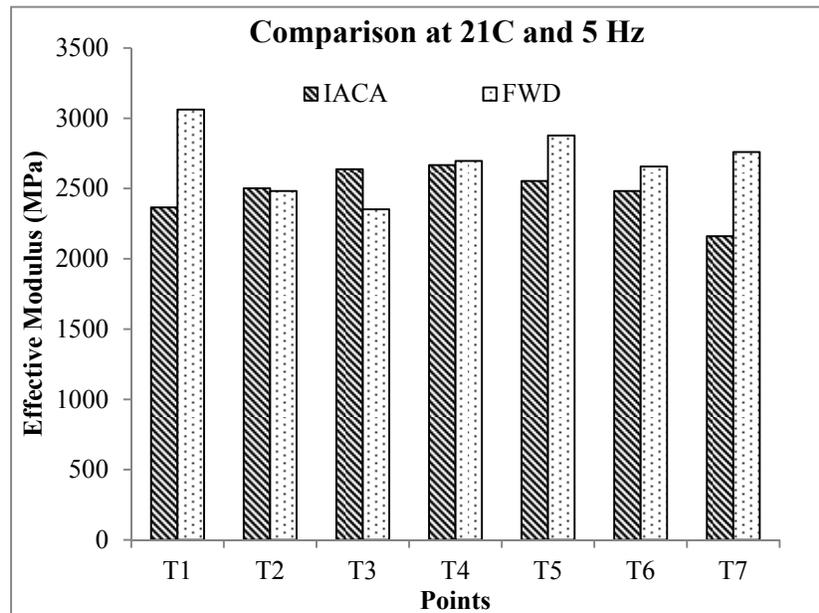
Figure 2 Comparison of Effective Modulus and FWD Modulus
