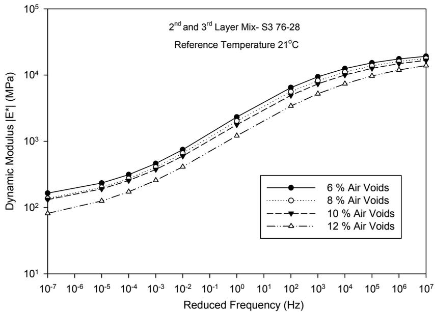
Figure 1 Master Curves for 2<sup>nd</sup> and 3<sup>rd</sup> Layers Mixes (S3 76-28)
