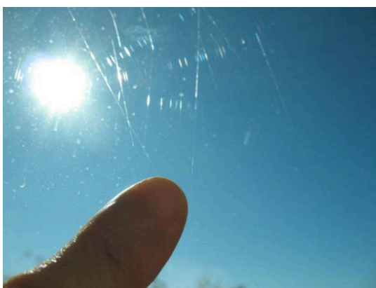
Figure 13. Combination of linear scratches and angel hair scratches observed in direct sunlight. (RCI 2010, with permission from RCI, Inc.).
