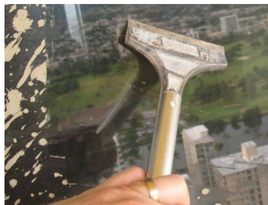
Figure 12. Tile scraper reportedly used to remove concrete patching debris from glass. (RCI 2010, with permission from RCI, Inc.).
