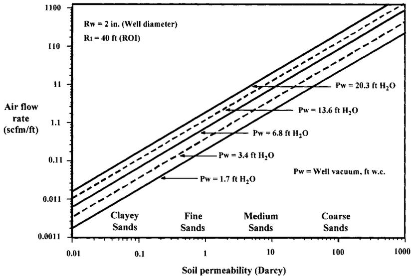
**Figure 8-3 Air flowrate versus soil air permeability and applied vacuum (US EPA, 1991d, Appendix E).**
