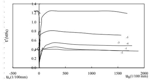
Figure 8 Stress-strain curve of shear test of structure plane (shear resistance/ residual strength)
