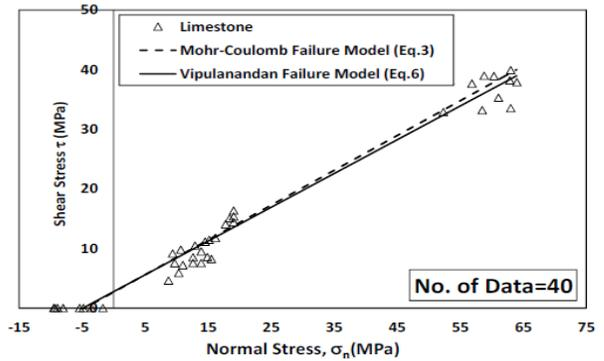
Fig. 6c. Failure shear and normal stress for limestone
