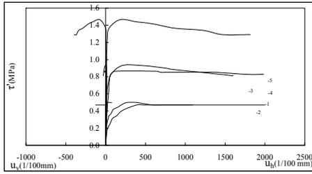
Figure 7 Stress-strain curve of shear test of structure plane (shear resistance cutting/peak strength)
