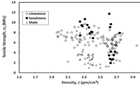
Fig. 4b. Variation of tensile strength with density for sandstone, shale and limestone
