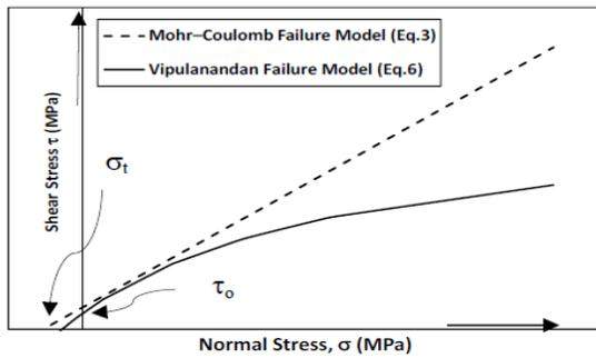
Fig. 5. Vipulanandan failure mode compared to Mohr-Coulomb model
