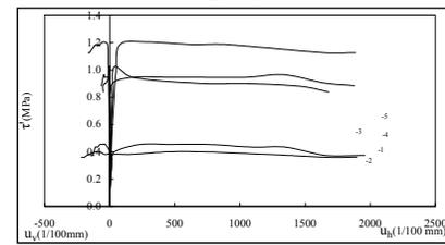
Figure 10 Stress-strain curve of on-site concrete / rock mass shear test (shear resistance/ residual strength)
