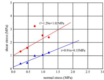
Figure 12 Shear strength curve of On-site concrete/rock mass shear test
