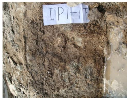
**Figure 6 Characteristics of shearing surface after shearing in the shear test point**
