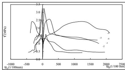
Figure 9 Stress-strain curve of on-site concrete / rock mass shear test (shear resistance cutting/peak strength)
