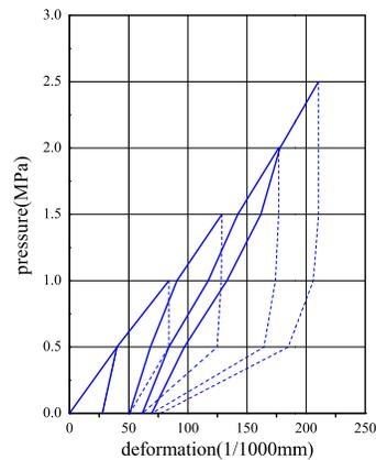
**Figure 4 On-site deformation test curve of Lilaitou reef rock mass (E<sub>0</sub>-2(V))**
