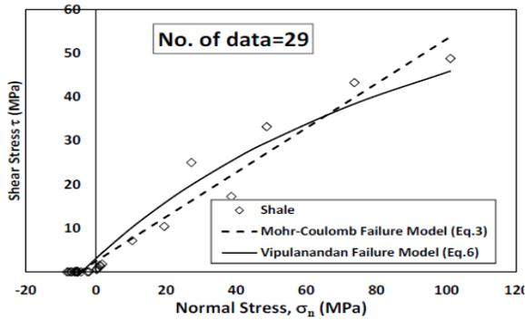
Fig. 6b. Failure shear and normal stress for shale
