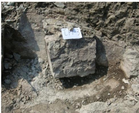
**Figure 5 Sample preparations before shearing in the shear test point**
