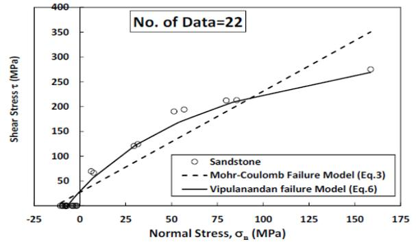
Fig. 6a. Failure shear and normal stress for sandstone
