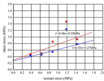
Figure 11 Shear resistance strength curve of shear test of controlling structural plane
