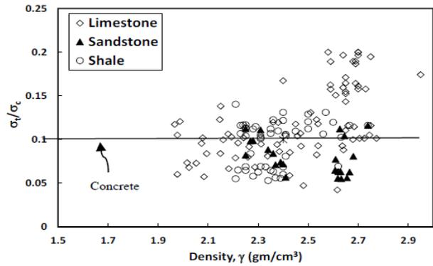
Fig. 4c. Variation of tensile/ compressive strength ratio with density for sandstone, shale and limestone
