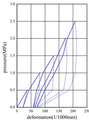
**Figure 3 On-site deformation test curve of Lilaitou reef rock mass (E<sub>0</sub>-1(V))**
