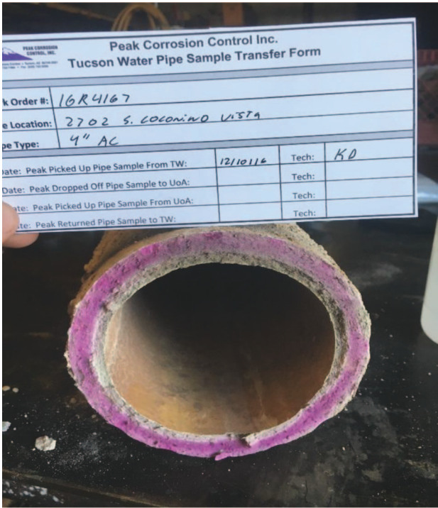
Fig. 9-7. Phenolphthalein dye test of asbestos cement pipe wall cross section Source: Courtesy of Tucson Water
