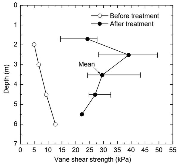
**FIG. 6. Vane shear test results before and after EK treatment.**
