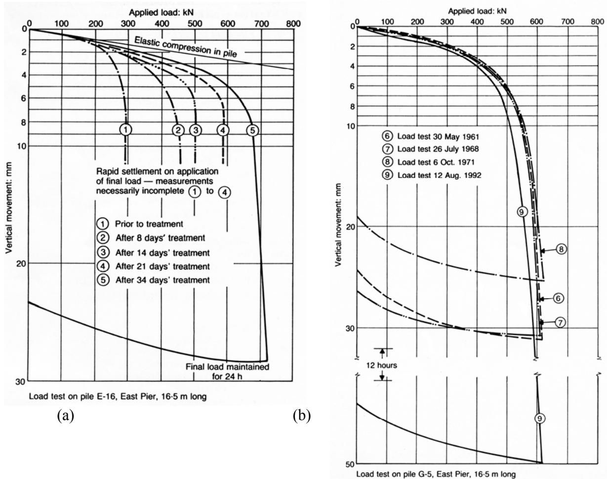
**FIG. 3. Pile load test results (Milligan 1995) (a) during EK treatment (b) after EK treatment.**
