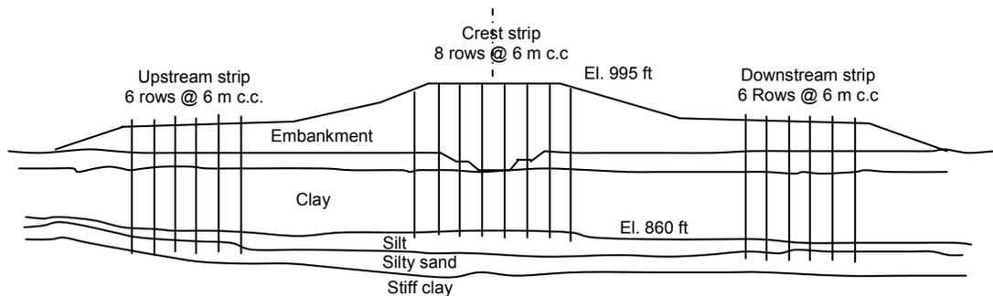
**FIG. 2. Section through electrodes (modified from Fetzer, 1967).**
