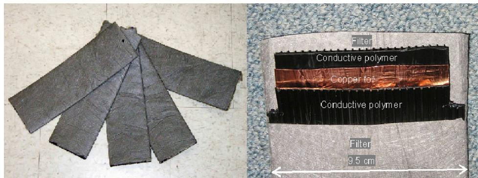
**FIG. 4. Electrical vertical drains (EVDs).**
