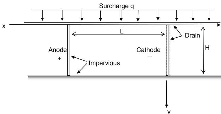
**FIG. 1. Schematic of electro-osmotic consolidation (modified from Shang 1998).**
