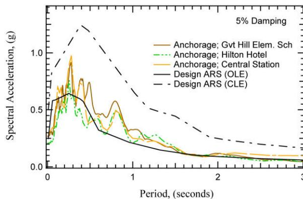
**Figure 15: ARS for M7.0 Earthquake**
