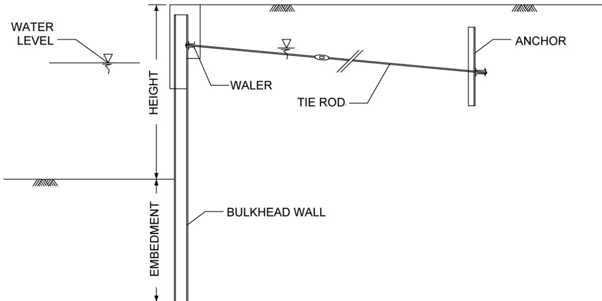
**Figure 1: Typical Anchored Bulkhead**
