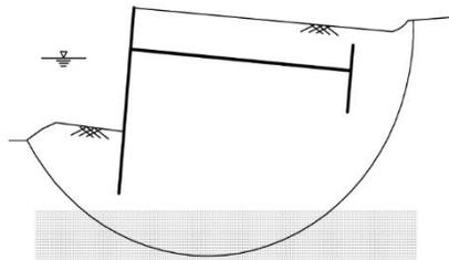
**Figure 3: Sketch of Global Stability Failure**
