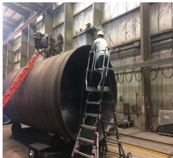
Figure 7. Steel Plates Welded into Cylinders
