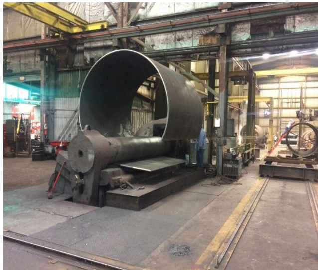
Figure 6. Steel Plates Being rolled
