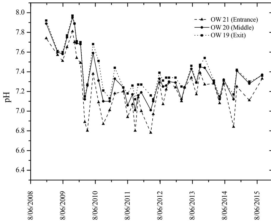
FIG. 7. pH along a centre-line of PRB (OW21-Entrance, OW20-Middle, OW19-Exit).
