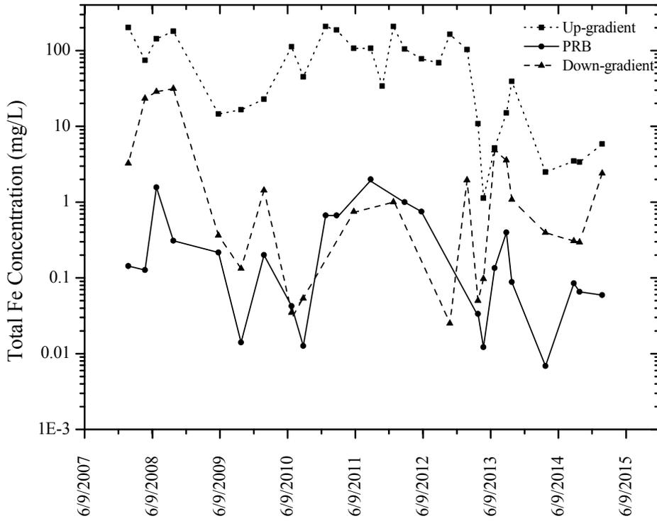
FIG. 6. Total Fe concentration in the up-gradient, PRB and down-gradient.
