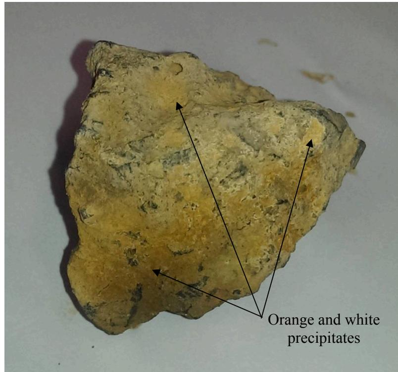
**FIG. 8. Recycled concrete sample exhumed from the entrance zone of PRB.**
