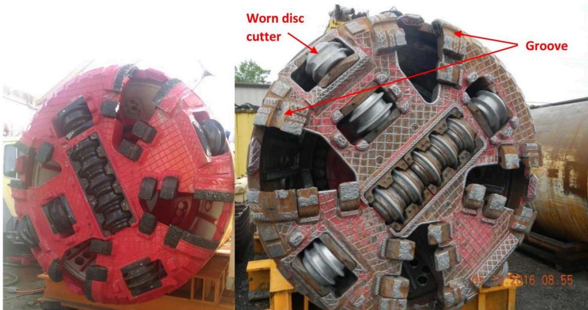
**Figure 2. MTBM Face Before (Left) and After (Right) First Microtunnel Drive**
