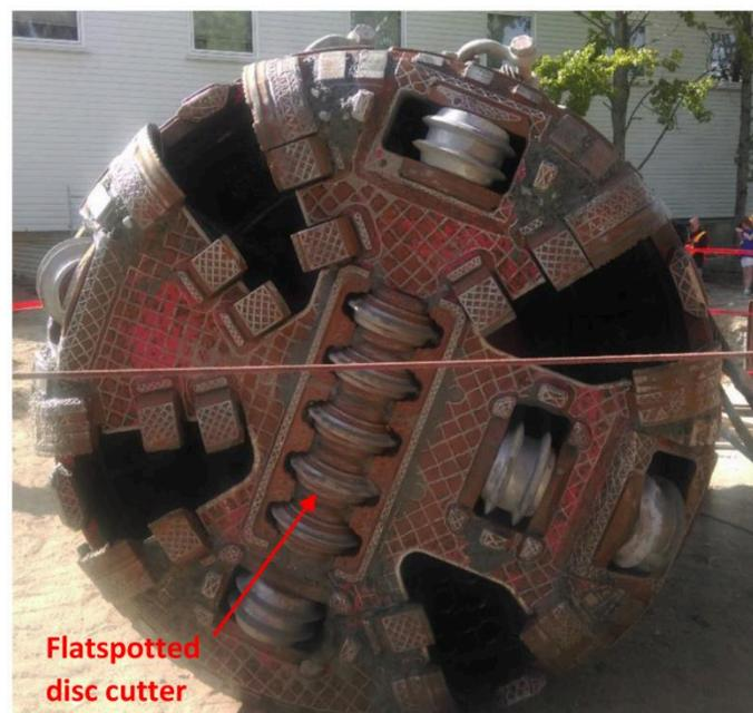
**Figure 4. Cutterhead upon Completion of the Second Microtunnel Drive**
