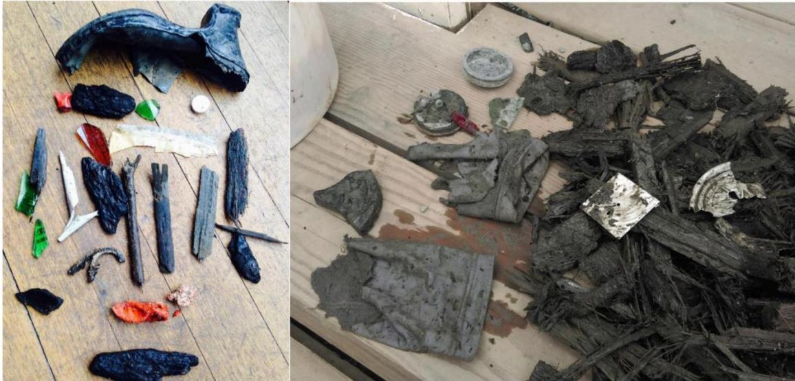
**Figure 3. Manmade Debris Encountered in Second Microtunnel Drive**
