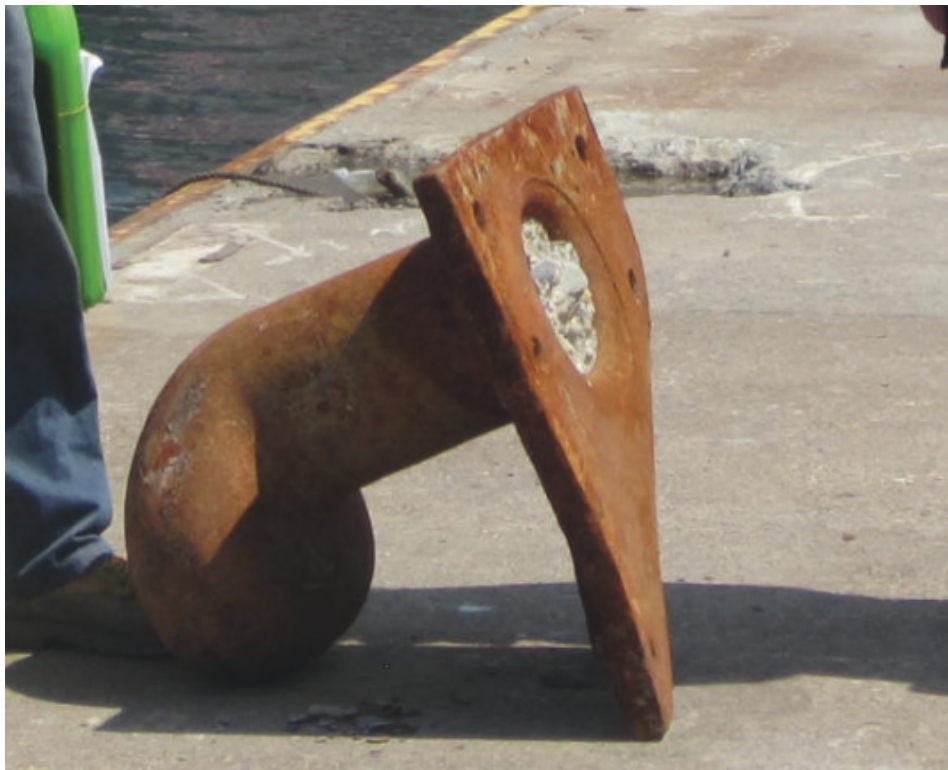
Figure 8-46 - Bollard with bent base plate at northern end of Location 5 wharf
