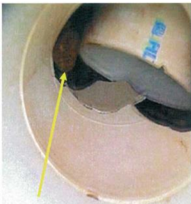
PHOTOGRAPH 2. Crushed Elbow at the Left End of the Spillway Stilling Basin Underdrain System. Arrow points to gravel observed outside the pipe. (Hawkins, 2010)
