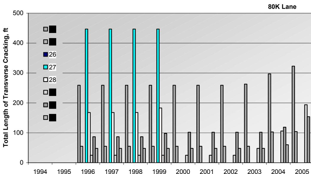
**Figure 5. Thermal Cracking Progression Over Time on Original LVR Cells**
