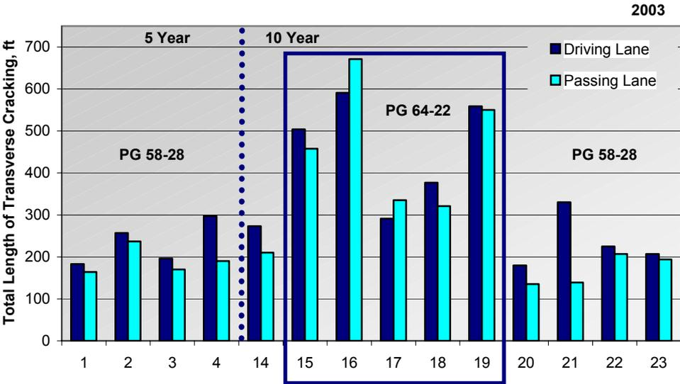
**Figure 3. Mainline Thermal Cracking by Cell (2003)**
