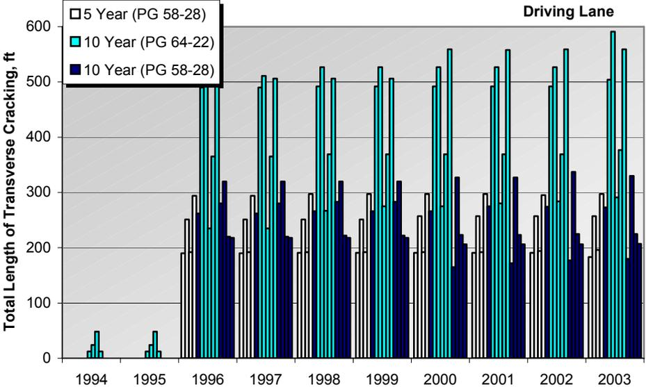
**Figure 2. Mainline Thermal Cracking History (Driving Lane)**
