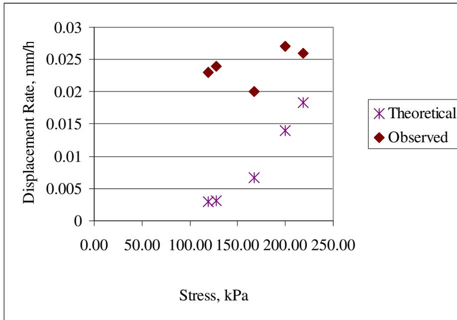
**Figure 9. Theoretical and observed displacement rates with stress**
