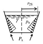
$r_{2S}$  is the radius at the fluid surface
